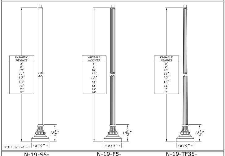
N-19-S5-\_\_\_ 5" dia. smooth shaft 8'-16' in height N-19-F5-\_\_\_ 5" dia. fluted shaft 8'-16' in height
