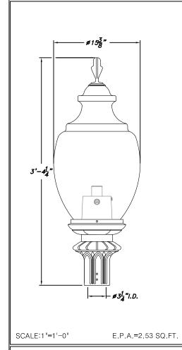
OPTIONAL CAST ALUMINUM FINIAL A-5015 GLOBE U.V. STABILIZED FROSTED OR WHITE POLYCARBONATE MOGUL OR MEDIUM 4KV BASED LAMP SOCKET MOUNTED TO BALLAST CAST ALUMINUM BALLAST HOUSING W/  $\oplus$ CANISTER HEAT DISSIPATION VENTS (2 @ 180°) CFL OR HID BALLAST CAPACITOR & STARTER (4) ½"-18x ¾" S.S. CONE POINT SET SCREW (4) 5"-18x 3" S.S. CONE POINT (4) ╬"−18x ¾" S.S. CUP POINT SET SCREW SET SCREW
