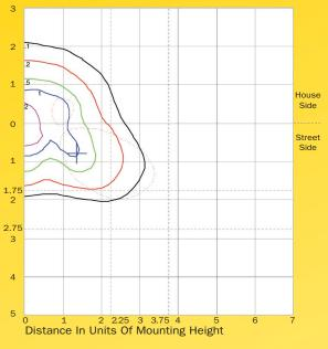
Values Based On 30 Foot Mounting Height 1/2 Maximum Candela Trace Shown As Dashed Curve
